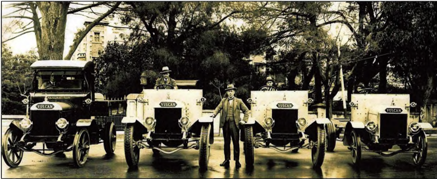
This fabulous period photo shows four Vulcans delivered to Australia. The centre trucks appear to have balloon tyres. I would like to get a lighting set with cradle brackets for my truck, they are probably CAV. Note the characteristic drop in the front axle.
