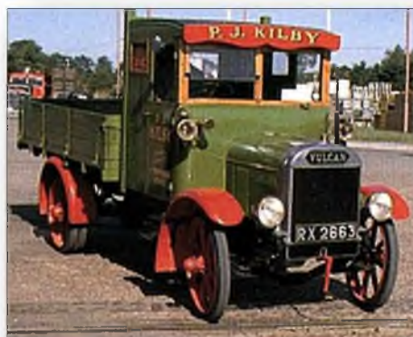
1927 Vulcan VSD 2-tonner powered by Vulcan's own design 4 cylinder petrol engine
