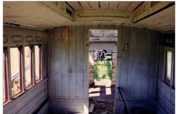
The interior had numerous coats of paint to remove which took months with heat guns and paint remover to reveal some very nice wood surfaces that we clear varnished
