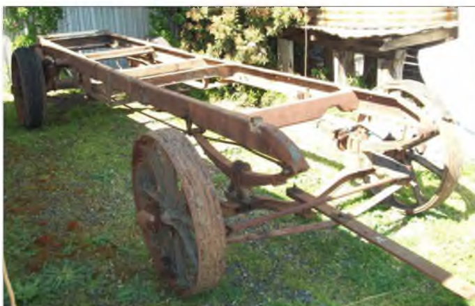
The trailer draw bar is connected in the centre of the axle as well as the steering ball joints to steer the trailer, which is fortunate as on some trailers the axle are welded fixed and a central pivot is used like a billy cart.
