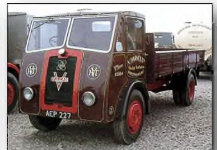
1948 Forward control Vulcan 6PF dropside truck with Perkins P6 engine.
