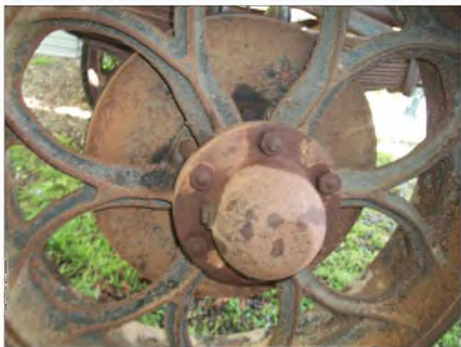
Complex wheel design compared to the front wheels. Large brake drums are no doubt adequate considering the slow speeds the truck would travel
