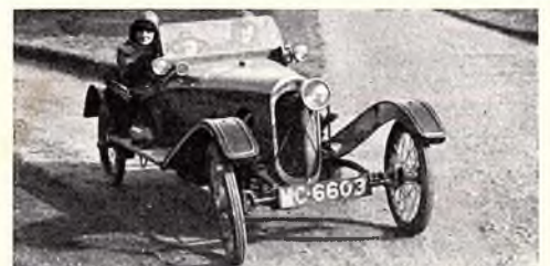
Year: 1919. Maker's H.P. and R.A.C. Rating: 8.7 h.p. Number of Cylinders: 2. Bore and Stroke: 84 x 98 mm. Engine Capacity: 1.1 litre. Valves: side or overhead. Wheelbase: 8' 6". Forward Speeds: 3. Final Drive Ratio: to choice. Tyres: 650 x 65. Illustration: 8.7 h.p.
